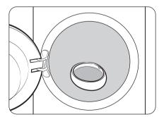
Pour the recommended amount of liquid or powdered detergent (specialty detergent) into the Aqua Pebble, and then put the Aqua Pebble directly into the drum. There are two guidelines inside the Aqua Pebble to indicate 50 ml (1.69 fl oz) and 100 ml (3.38 fl oz). Do not exceed the 100 ml line.
