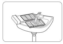
**4.** Remove lint on both inner and outer filters. Then, wash the filters in running water and completely dry the filters in a shade.
