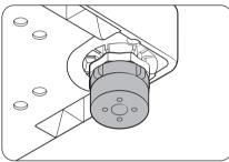
With the leg ring in place, use the leveling leg to adjust the height of the washer.
