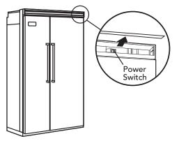
**IMPORTANT:** Be sure the power on/off switch is in the on position after cleaning or changing light bulbs.
