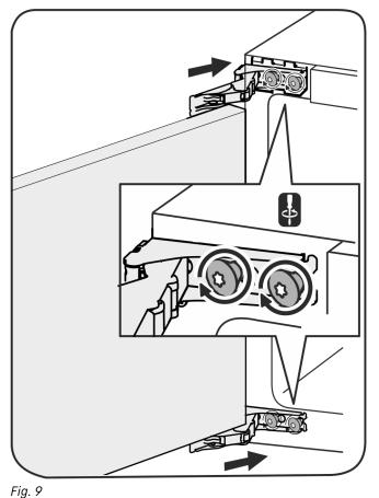
Fitting the door again: Reattach the door to the hinges and tighten the screws.
