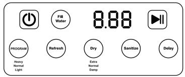
**On/O ffPower icon** () - Powers on the Steam Dryer Closet. All the selections on the Control Panel illuminate.
