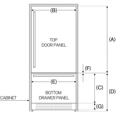
**NOTE**: These specifications assume a standard toe kick height of 4". For different toe kick heights, adjust C accordingly.
