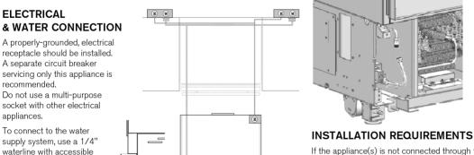
If the appliance(s) is not connected through the side profile trims to secured cabinetry, anti-tip brackets must be installed. The max weight for the cabinet panel is 35 lbs (16kg) for the refrigerator door and 20 lbs (9kg) for the freezer door. For a flush installation, cabinet panels should not be thicker than 15/16".
