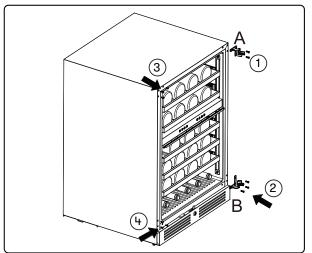
4. Unscrew 6 screws from hinge 1 and 2 and 6 black decorative nails from 3 and 4 on the body of the unit. Reinstall the hinge, marked A, to the lower left corner. Reinstall the hinge, marked B, to the upper left corner. Then reinstall the 6 black decorative nails to the right side.
