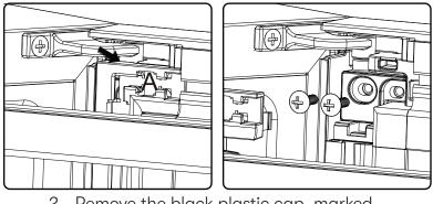
Remove the black plastic cap, marked A, at the upper right corner of the door and the cap, marked B, at the lower right corner. Remove 2 screws from both the upper and lower hinge.
