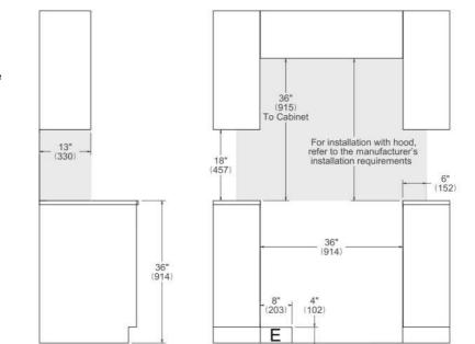
NOTE a. Electrical Connection b. Gas Connection
