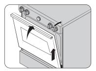
**5.** Lift door up and out until the hinge arm is clear of the slot (Fig. 2).
