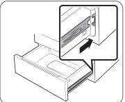
**4.** Put the drawer in the roller guides on either side, and then snap the clips into place.
