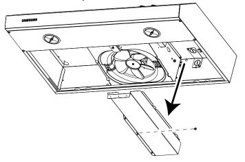
3. Using a flat head screwdriver, remove the appropriate power supply
