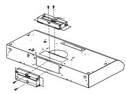
1. Using (2) short Phillips head screws, install the 31/4" x 10" (8.3 x 25.4 cm) rectangular damper over the top or rear vent knockout removed in previous step.
