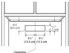
3. Use saber or keyhole saw to cut a rectangular opening in the wall for the vent
