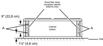
1. If cabinet has recessed bottom, add wood filler strips on each side. Install 4 flat head wood screws with washers and nuts to attach filler strips in locations shown.
