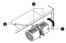
Attach one or two blower unit mounting screw(s) **1**. Attach the cover plate **2** on the back. Attach the blower plate 3 to the microwave oven. Attach one or several blower plate mounting screw(s) 4. Attach the cover plate **2** on the blower plate and attach the screw 7
