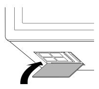
**4** To reinstall the grease filter, insert the back of the filter, push the filter toward the back, and lift the filter up into place.
