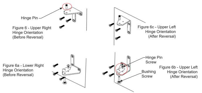
5. Using a 5/32" Hex Key, remove the Upper and Lower Hinge Brackets from the door (Fig. 7), saving all components. Remove black plugs from opposite side of door. flip the Upper Hinge Bracket and reattach the Hinge Bushing (Fig. 7) and screw into place on the opposite side of the door (where plugs were removed). Remove the Cam Closer from the Lower-Hinge Bracket (Fig. 7) and attach it to the opposite side (Fig. 7b).
