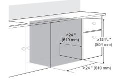
2 To allow for proper clearance of plumbing and electrical, use the template included with the literature to determine the clearance on the side of the cabinet where the cabinet meets the back wall. Using a 2 1/2" diameter hole saw, drill a hole in the target area as shown on the template.
