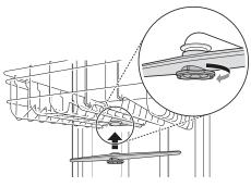
**7** After assembly, make sure that the spray arms rotate freely.
