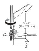
Pull the existing wires through the openings in the junction box. Tighten 2 screws 4 to reassemble the junction box in the appliance.
