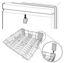
• Press the tab to remove the cable tie by hand. Cutting the tie with a knife or scissors may damage the rack or the silverware basket.
