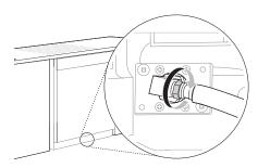
**3** Slide the water supply line back through the channel, pulling gently from inside the cabinet to make sure the line is not kinked, pinched, stressed or crushed.
