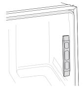
Make sure that the gap between the tub walls and the door liner is the same on either side.
