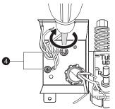
8 Pair the white, black, and green wires to the matching colored wires from the dishwasher. Then twist on the provided wire nuts **9** tightly to connect the corresponding wires.
