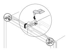
**2** Bend the tabs on the brackets to secure them to the frame using a pair of needle nose pliers.
