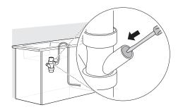
**2** Attach the drain hose to the waste tee with the hose clamp provided. Move the clamp into position and tighten it with a flat-blade screwdriver.
