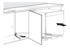
**5** Remove the tape from the water supply line and the electrical cable.
