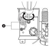
8 Pair the white, black, and green wires to the matching colored wires from the dishwasher. Then twist on the provided wire nuts **5** tightly to connect the corresponding wires.
