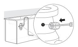
**2** Remove the knockout plug **1** from the disposal.
