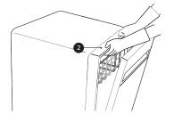
**1** Align the dishwasher with the opening. Make sure the water supply line and electrical cable are in the correct positions to slide into their channels properly.
