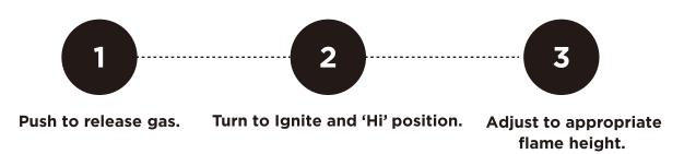
To light the surface burners, push and turn the appropriate control knob counter clockwise to a "Hi" position. You will hear a clicking noise – the sound of the electric spark igniting the burner.
