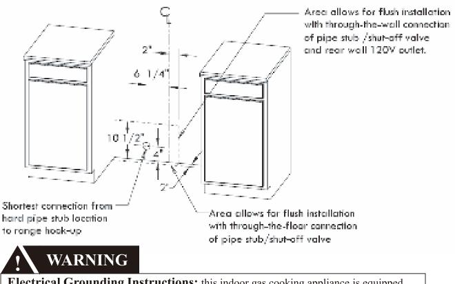
**Electrical Grounding Instructions:** this indoor gas cooking appliance is equipped with a three prong (grounding) plug for your protection against shock hazard and should be plugged directly into a properly grounded three pronged receptacle.
