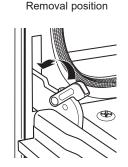
Rest notch on bottom edge of hinge slot
