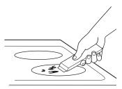
The ceramic cooktop scraper and all recommended supplies are available through our Parts Center. See the Accessories and Consumer Support sections at the end of this manual. **NOTE:** Do not use a dull or nicked blade.
