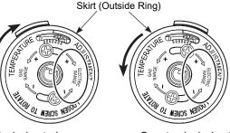
Clockwise to Increase Counte Temperature Decrease (Shown at highest setting) (Shown at Back of OVEN TEMP knob
