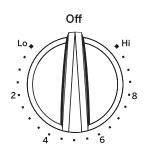
At both **OFF** and **HI** the control clicks into position. You may hear slight clicking sounds during cooking, indicating the control is maintaining your desired setting.
