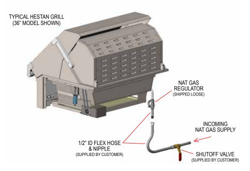
Your Hestan grill for use with Natural Gas is supplied with its own regulator which <u>MUST</u> be installed. If this regulator needs to be replaced, use only the type specified by Hestan for this appliance.
