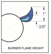
There should be no excessive noise or flame lifting. If any of these conditions exist, remove the burners and check if dirt, debris, spider webs, etc., are blocking the air shutter or burner ports. Proceed with air shutter adjustment if necessary.
