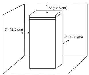
Place the appliance on a flat level surface, leaving 5 inches (12.5 cm) on either side and at least 5 inches (12.5 cm) between back of appliance and the wall.
