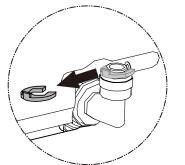
2. Take out the soft pipe from the freezer drawer, insert it into the connector and push it to the end, the soft pipe should be ¼ inch (6.35mm) in external diameter.
