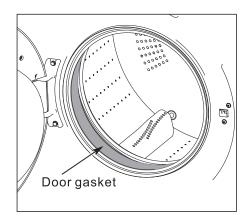
Clean the door gasket once a month to prevent buildup of dirt in the door gasket.
