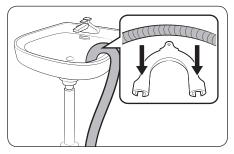
Height difference between the installation location of the washing machine and the drainage point: Minimum 24", and Maximum 40".
