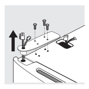
5. Lift to remove the door and place on a soft pad.
