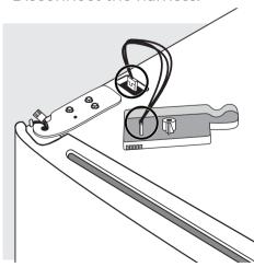
4. Unscrew 3 bolts and remove top hinge.
