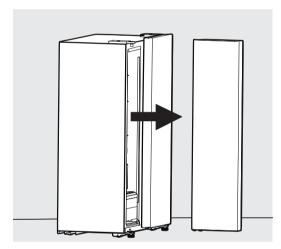
6. Repeat for the other door. After the appliance is in position, reinstall the doors using the reverse procedure.
