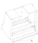
15. Only for ETRXXXXX hood models attach hood insert rear bracket support with 4 - 3.5 x 9.5 mm screws on the back.
