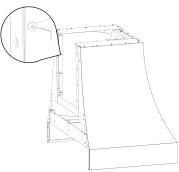
18. Lift the hood cabinet beneath the motor housing. Insert the cabinet pins into the vertical support slots. Once the eight pins are already inserted, the cabinet stands hanging.
