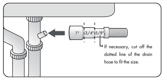
4. Slide the provided hose clamp over the end of the drain hose. Attach the drain hose to the sink connector, slide the hose clamp to the end of the hose, and then tighten the hose clamp.
