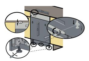
If height of the enclosure is  $32 \, 1/8$ " (816 mm) to  $34 \, 1/8$ " (867 mm), use the short leg supports as shown in the figure above.
