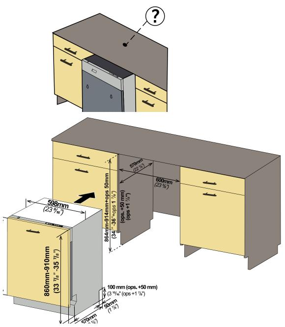
NOTE: Since kitchen layouts vary, ZLINE recommends consulting with a professional installer to verify cabinet dimensions before installing the appliance.
