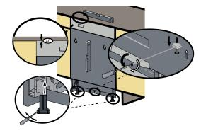
If the height is above  $34 \, 1/8$ " ( $867 \, \text{mm}$ ), use the long leg supports as shown in the figure above.
