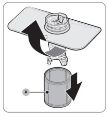
4. Disassemble the micro filter (A).
