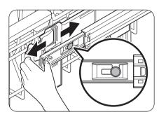
**4.** Slide the upper rack so that the shaft is positioned at end of the rail bracket.
