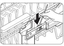
1. Push the hook on the rail holder (on left and right sides).
