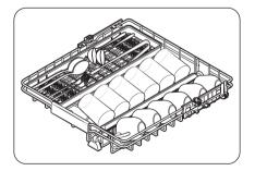
You can load flatware on the left side of the rack and cups and glasses (that are shorter than 6 inches) on the right side of the rack.
