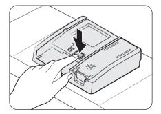
1. Press the button on the detergent compartment cover to open the detergent compartment cover.
