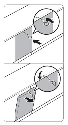
If you are unable to use the Auto Open Door function because of a power failure or other reasons, use the provided Emergency handle to open the door manually.
