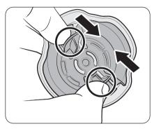
6. Remove the coarse filter cap.
