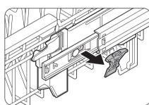
**2.** Remove the rail holder from the rail (on left and right sides).
