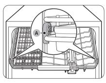
1. Facing the dishwasher, pull out the 3rd rack fully and slightly push back until the **handles (A)** line up with the front side of the rack.
