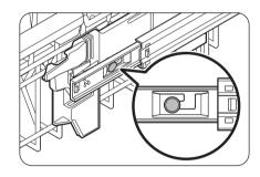
3. Check the position of the shaft on the rail bracket.
