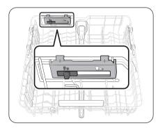
You can use the upper rack's guide tines to load items onto the upper rack in various ways. Move the slider to the right or left to adjust the guide tines suitable for loading the following items.
