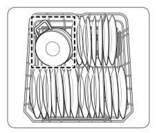
For more effective cleaning, load large items into the Storm Wash+ area on the left side of the lower rack (Dotted zone).
