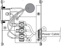
The dryer is now ready to be plugged into the 3-wire receptacle of the proper rating.
