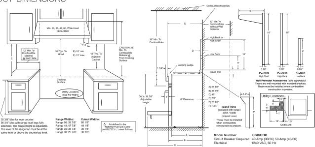
GAS REQUIREMENTS: 1/2" NPT gas connection. Minimum gas supply is 7" water column for natural gas and 11" for propane. Operating pressure at the manifold is 5" water column for natural gas and 10" for propane. All units include a gas regulator. The installer must provide a shut-off valve at the rear of the appliance with easy access to shut off the gas for service. High-altitude kits and gas conversion kits are available through the Capital parts department.
