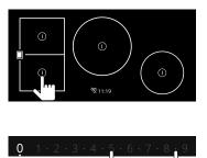
2 Selecting a power level turns on the cooking zone. The cooking zone indicator remains lit and the power level is stored.
