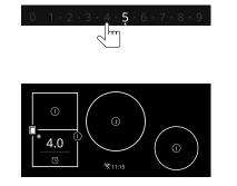
2 Press the desired level in the **Power Levels** popup. If no selection is made, the Power Levels popup disappears after 3 seconds and the power level remains the same.
