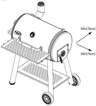
30in[76cm] minimum clearance from any combustible surfaces
