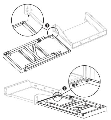
**STEP 12** Use two (2) M5x15 bolts [c.] to attach the right rotation bracket to the right table.
