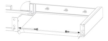
$\underline{\textbf{STEP 15}}$  Screw two (2) M6 step bolts [f.] into the top holes of the left side shelf.
