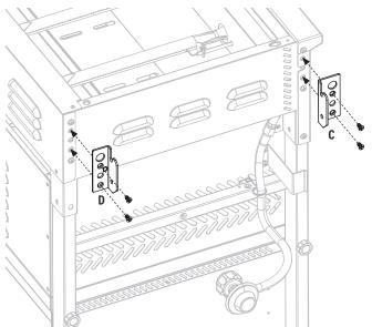
**STEP 08** Use three (3) wing nuts [e.] to attach three (3) washers [h.], three slotted washers [i.], and three (3) side shelf pegs [b.] to the right side shelf.
