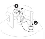
**STEP 02** Hold the regulator in a straight line with the Type 1 valve outlet so as not to cross thread the connection.
