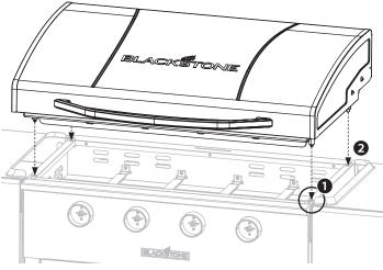
• Place the two front pins into the front locking holes and push the griddle top back.
