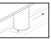
**STEP 23** Hang the grease cup with grease cup liner in the slot at the back of the griddle body.
