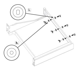
**STEP 09** Use three (3) wing nuts [**e**.] to attach three (3) washers [**h**.], three slotted washers [**i**.], and three (3) side shelf pegs [**b**.] to the left side shelf.
