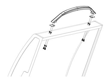
**STEP 22** With the help of another person, place the griddle top and hood on the main body by aligning the 4 pins to the holes of the body.
