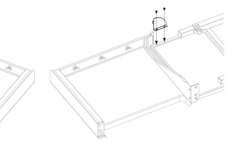
$\underline{\text{STEP 14}}$  Screw two (2) M6 step bolts  $[\mathbf{f.}]$  into the top holes of the right side shelf.
