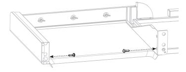
**STEP 16** Hook the right side shelf's upper step bolts on the side shelf brackets. Use two (2) M6 step bolts [f.] to secure the side shelf to the side shelf brackets.
