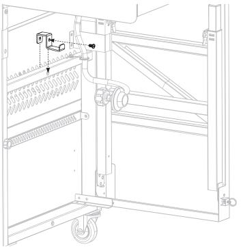
**STEP 20** Use one (1) M6x12 bolt [a.] to attach the LPG support to the left leg assembly.
