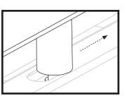
**STEP 04** Use the two (2) M6 bolts pre-installed in the handle to attach the handle and bezels to the hood.
