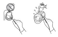
5 To reassemble the vent cover, place it over the supply tube in the same orientation as it was removed (about 2 o'clock). Turn the cover counterclockwise until it clicks into place.
