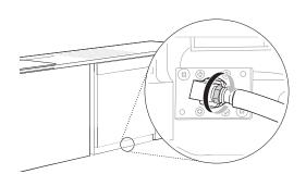
3 Slide the water supply line back through the channel, pulling gently from inside the cabinet to make sure the line is not kinked, pinched, stressed or crushed.
