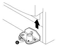
**4** Place the door, inside facing up, on a non-scratching surface.
