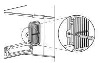
**3** Press on the hooks at the air filter and then take it out.
