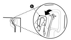
3 Pull out the water supply lines ♥ at the top of the refrigerator. Disconnect all the wire harnesses ③. Unscrew the ground wire ⑨.
