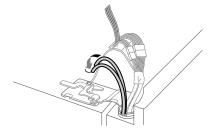
5 Hold the water supply connection and gently push in the collet **③** to connect the water supply lines as shown. Insert the tube at least 5/8 inch (15 mm) into the connector. Insert the clip on the joint to fasten the tubes in place.
