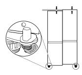
**1** Open the door and use the wrench to loosen the keeper nut by turning it to the left.
