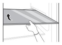
3 Make sure the door is open as far as possible before pulling the shelf forward to remove it. If needed, have an assistant to fully open the door while you pull out the shelf.
