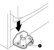
2 Fit the hinge ② over the hinge lever latch ③ and slot it into place. Rotate the lever ④ clockwise and fasten the hinge.
