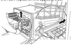
To replace the rack, place the back rack supports behind the rear hooks and pull the rack forward to snap the supports into the hooks. Then align the front rack supports with the front hooks and push the front of the rack down to snap the supports into the front hooks.
