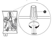
Wrap electrical tape **6** around each connection.
