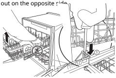
To remove the back rack supports from the rails, hold a side rail with one hand, lift the front of the rack, and firmly push the rack back to snap the support out of the hooks in the rear. Repeat on the opposite side.
