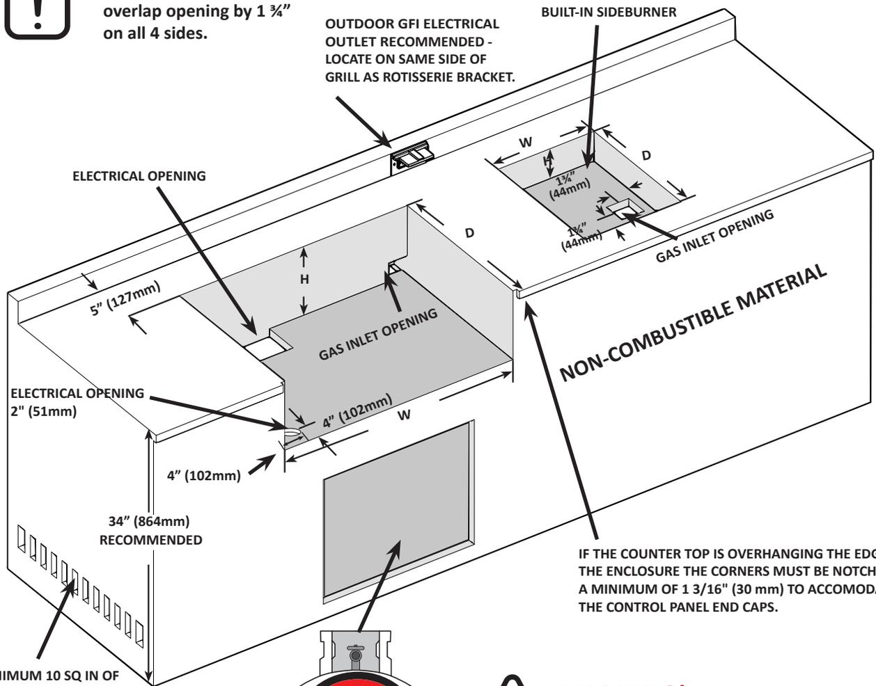
IF THE COUNTER TOP IS OVERHANGING THE EDGE OF THE ENCLOSURE THE CORNERS MUST BE NOTCHED A MINIMUM OF 1 3/16" (30 mm) TO ACCOMMODATE THE CONTROL PANEL END CAPS.
