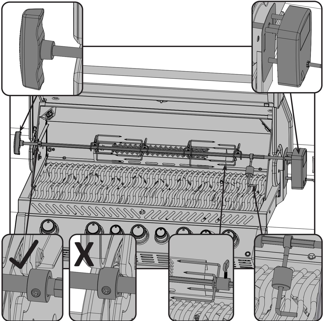
Ensure stop bushing is tightened on the inside of hood casting.
