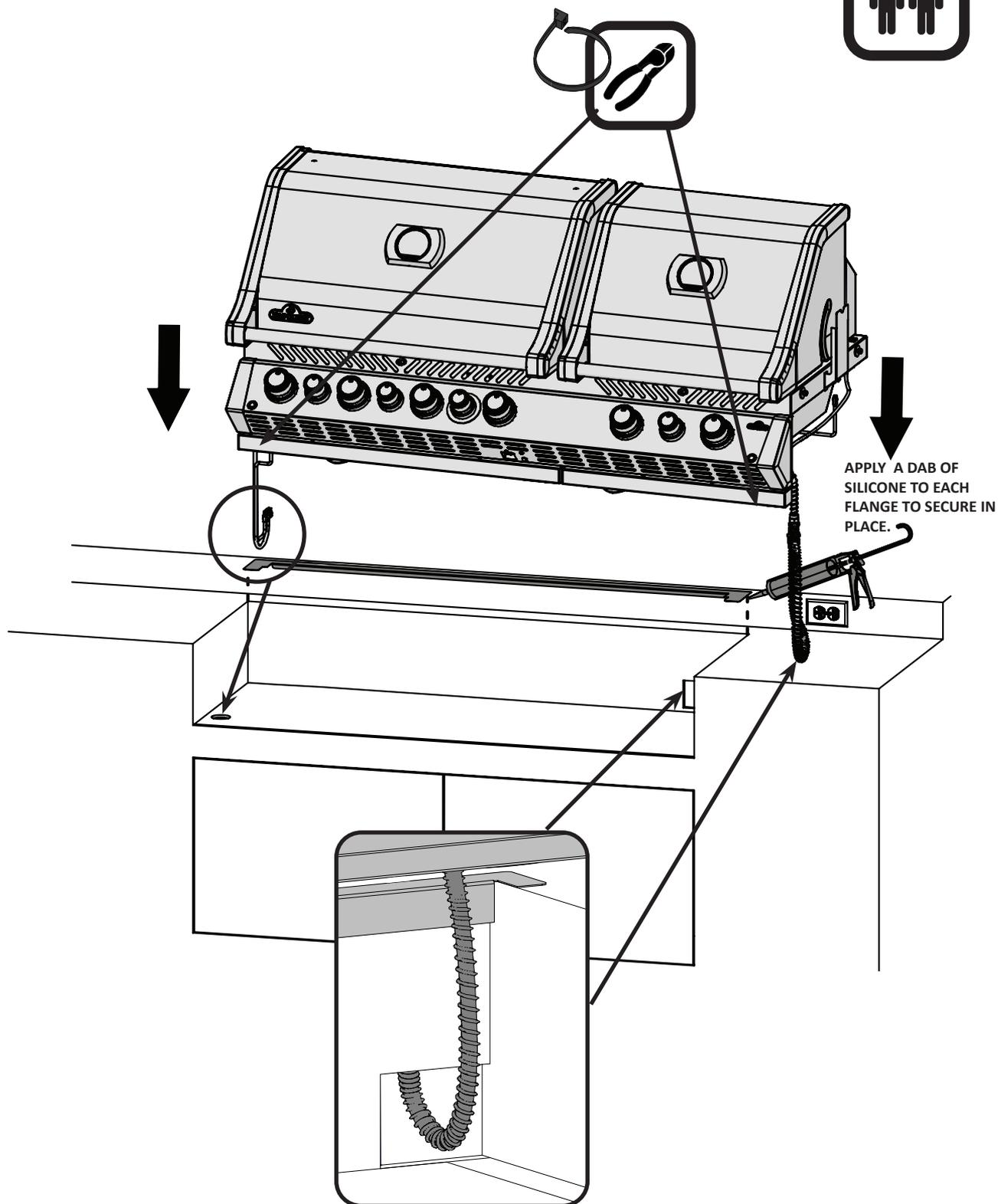
APPLY A DAB OF SILICONE TO EACH FLANGE TO SECURE IN PLACE.
