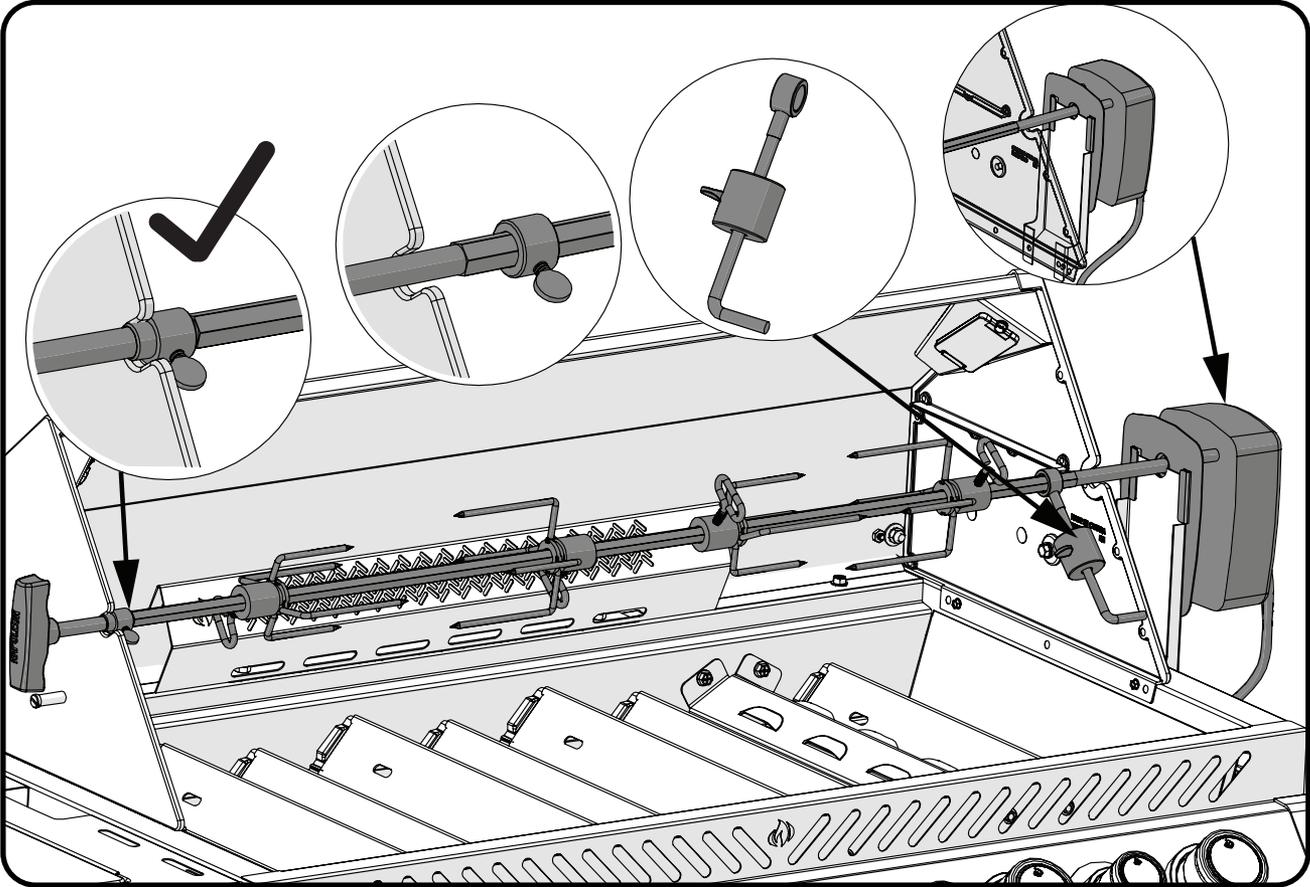
Ensure stop bushing is tightened on the inside of hood casting.
