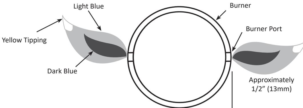
**Burner:** The burner is made from heavy wall 304 stainless steel, but extreme heat and a corrosive environment can cause surface corrosion to occur. This can be removed with a brass wire brush.
