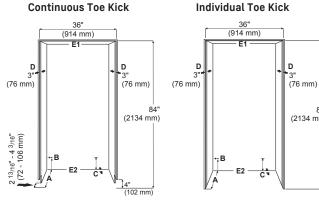
Cabinet depth frameless installation style = 25" (635 mm) Cabinet depth inset installation style = 25" (635 mm) + panel thickness
