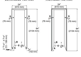
Cabinet depth frameless installation style = 25" (635 mm) Cabinet depth inset installation style = 25" (635 mm) + panel thickness
