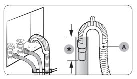
(\*): Min. 6 in. (152 mm), Max. 8 in. (203 mm)
