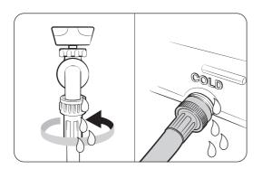
**5.** Open the water taps, and check for leaks.
