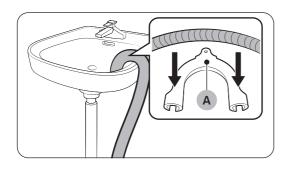
**3.** Route the drain hose to the drain system.
