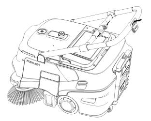
When you need to interact with the screen, there are two options: you can either open the screen protector and directly interact with the screen, or detach the screen from the robot and operate it either by holding it in your hands or by attaching it to the handle.
