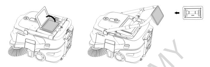
\* The robot handle and the screen are designed to be detachable.
